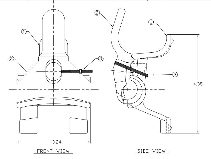
BODY & KEEPER - DUCTILE IRON, 654512 FINISH - HOT DIP GALVANIZED PER ASTM A153 MOUNTING BOLT - 5/8"
